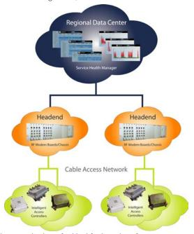
intelligent management of real-time monitoring of critical fault and performance indicators and correlation of RF, IP and QoE level information, including continuous path and upstream ingress monitoring and analysis. This intelligent management of the HFC network and services is also uniquely combined with the industry's only managed ingress suppression technology − Proxilliant's Dynamic Ingress Blocking™ technology − to eliminate the propagation of quality-eroding ingress.
